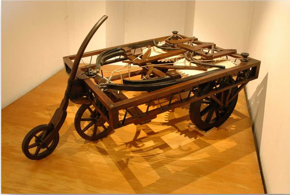
Drawing of a pre-programmed clockwork cart by Leonardo Da Vinci, circa 1478 Had it been built, this cart would have been powered by large coiled clockwork springs, propelling it over 130 feet. The clever control mechanism could have taken the vehicle through a predetermined course.
